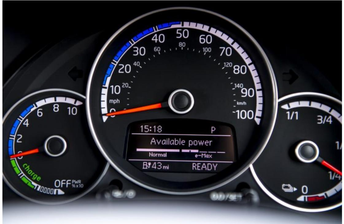
instruments for road-speed/ trip distance and flanked by sophisticated, charge meter and capacity gauges directly in front of the driver.
