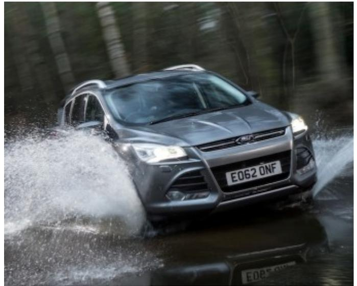
The all-new roomier Ford Kuga introduced at the start of this year has continued their engine down-sizing policy for better fuel economy and lower CO2 emissions and replaced the aging 2.5-litre engine with their latest technology 1.6-litre EcoBoost four cylinder turbocharged petrol engines with power outputs of 148 and 177bhp.
