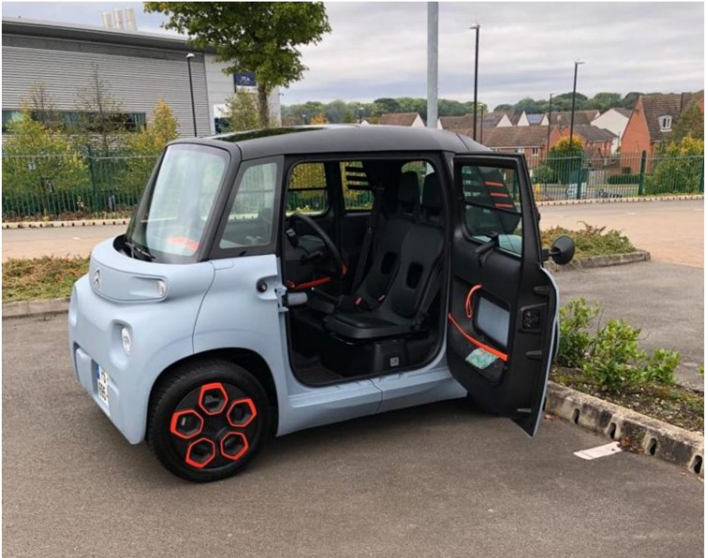
It's built only in left-hand-drive for the purpose of being an inexpensive city car and in France it retails for under €7,000 which gets you a two-seater with 6kW motor, 5.5kWh battery which recharges from its on-board tether in three hours and gives a 46 miles range with maximum speed of 28mph.
