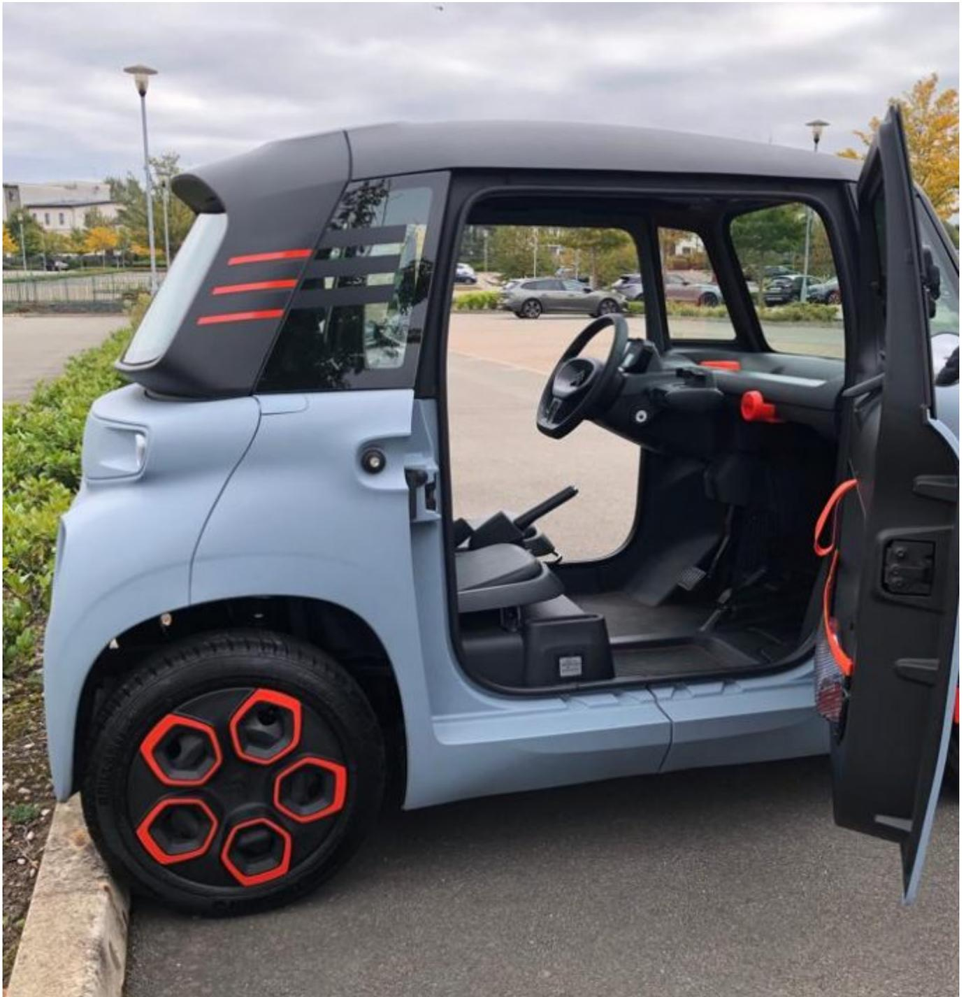
Access is excellent if a little different for most drivers using the so-called 'suicide-door' opening on the left hand side but passengers get a front hinged door. It does mean the
