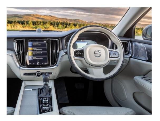
Inside, the new minimalist modern-day Volvo design theme continues. The Sensus 9.0-inch touchscreen control system allows the fascia to be largely free of buttons and switches. A 12.3-inch active digital driver's information screen fills the instrument binnacle.
