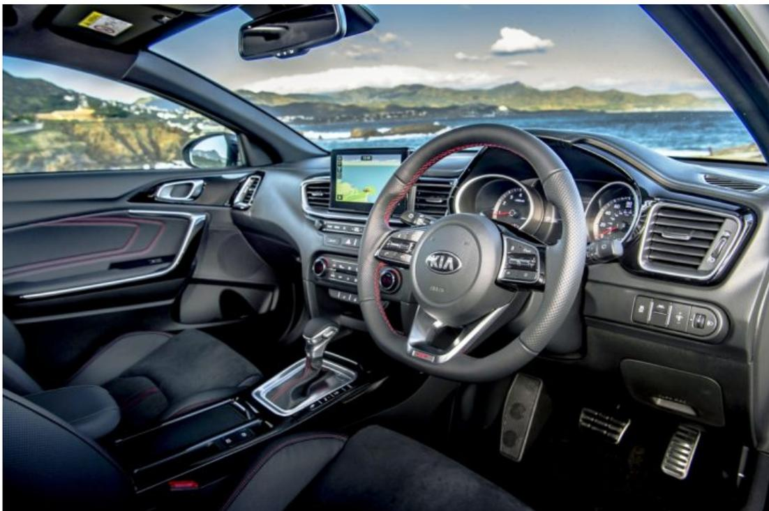
The sports seats of the ProCeed are lower in the body which offsets the potential loss of headroom. The lower roofline also means the side windows are shallower which restricts side
