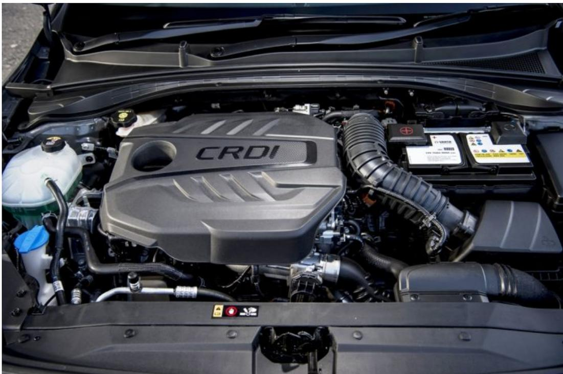
The GT-Line uses the latest Euro-6d-Temp emission regulations engines. These are a 1.4 T-GDi 138bhp turbo petrol with manual/auto gearbox options, the new 1.6 CRDi 134bhp
