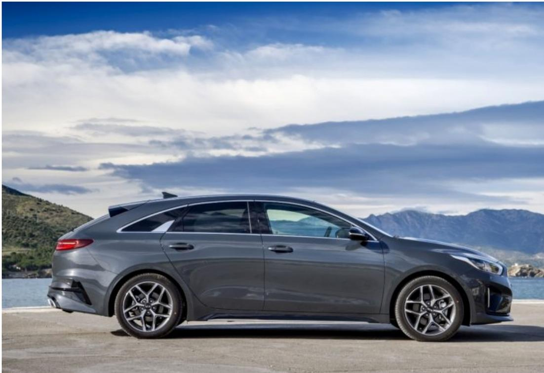
The downside of the ProCeed's styling is the steeply forward sloping tailgate window which restricts the load carrying height at the very rear of the boot space.
